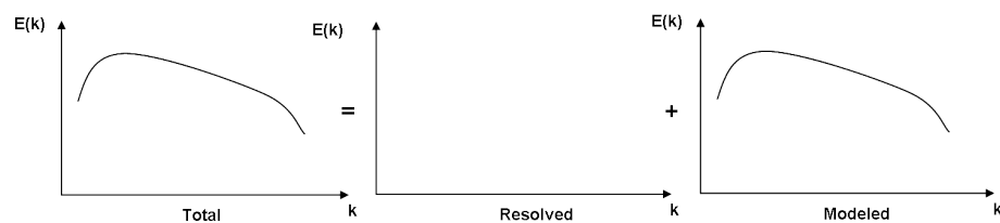
Figure 1.6: Schematic drawing of the resolved and modeled energy spectrum in RANS.
