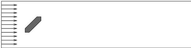
The flow in a channel hits a tilted plate. At the left boundary, the fluid inflow has a constant velocity profile ( $u = 1.0, v = 0.0$ ), while at the upper and lower boundaries no-slip conditions are imposed.
