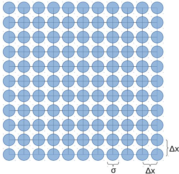
Figure 1: Particles (blue disks) are initialised on a grid with equidistant mesh size  $\Delta x$  in all spatial directions. For sake of simplicity, the two-dimensional case is shown.
