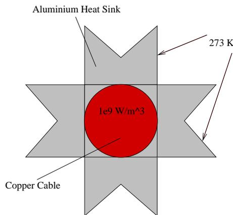
a) Build the heat sink geometry.
