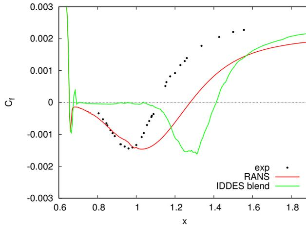
Figure 2: Space and time-averaged skin friction coefficient  $C_f$  for the 2D wall-mounted hump. The origin  $x = 0$  is placed at the beginning of the hump. The scenario was experimentally examined in [7]. The stabilization-blended improved delayed DES technique predicts the recirculation length better than a simple SST RANS model but mispredicts the separation point.
