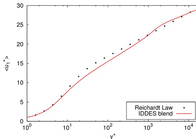
Figure 1: Time and space-averaged velocity profile in streaming direction  $\langle u_1^+ \rangle$  for the turbulent channel at  $Re_\tau = 18000$ . We compared the stabilization-blended improved delayed DES with the Reichardt correlation. The grid consisted of  $81 \times 125 \times 61$  nodes.
