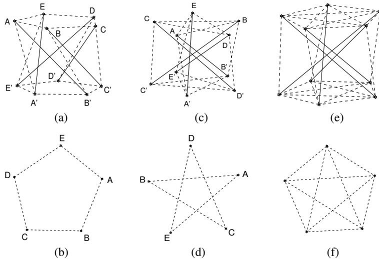
Figure 1: Example of a 5-plex with the standard connectivity  $j = k = 1$ : (a), (c) the two possible geometrical configurations with  $p = 1$  and  $p = 2$  respectively; (b), (d) constituent polygons of (a) and (c), respectively; (e), (f) structures corresponding to (c) and (d) with a stabilizing ring.
