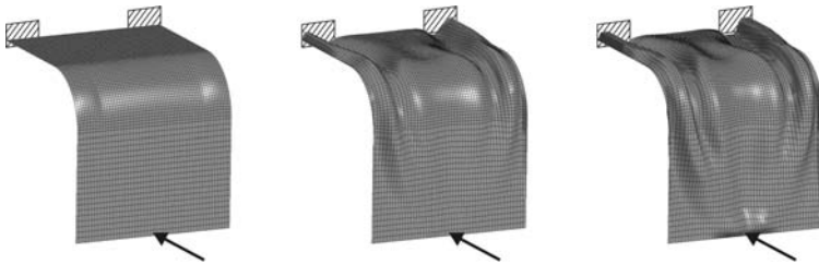
Fig.4: Shape optimization of a cantilever shell
