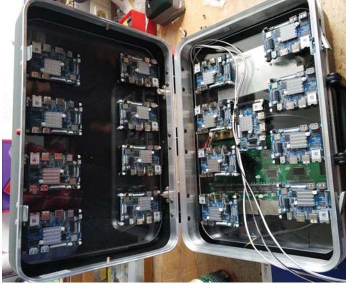
Figure 3: The Raspberry Pi Suitcase Cluster: A cluster consisting of Raspberry Pi computers for testing and presenting of the All-Scale architecture.
